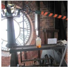
Showing the tower extending up from the clock mechanism, connected to the shaft, leading to each face mechanism. The shafts are wound with tape to draw the winder's awareness to the shafts to prevent head bumping and shaft damage.
